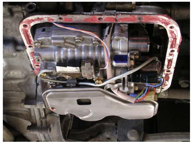
Fig.7. The primary hydraulic pressure sensor
