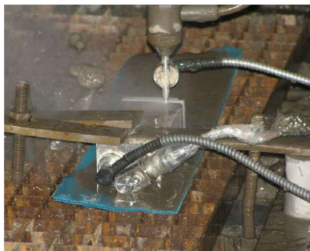
Fig. 1 Diagnostic measurement of vibrations in the evaluation of the impact of focusing tube wear during abrasive waterjet cutting of aluminum
