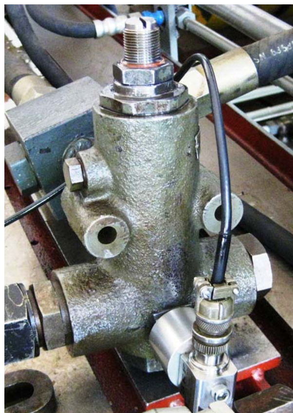
Fig. 1 Pressure valve PVV-25 and accelerometer with magnetic adapter
