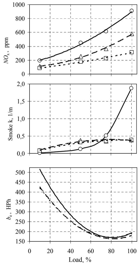
**Figure 7.** Comparison of load characteristics of 4 cylinder turbocharged diesel engines with different CCs.
