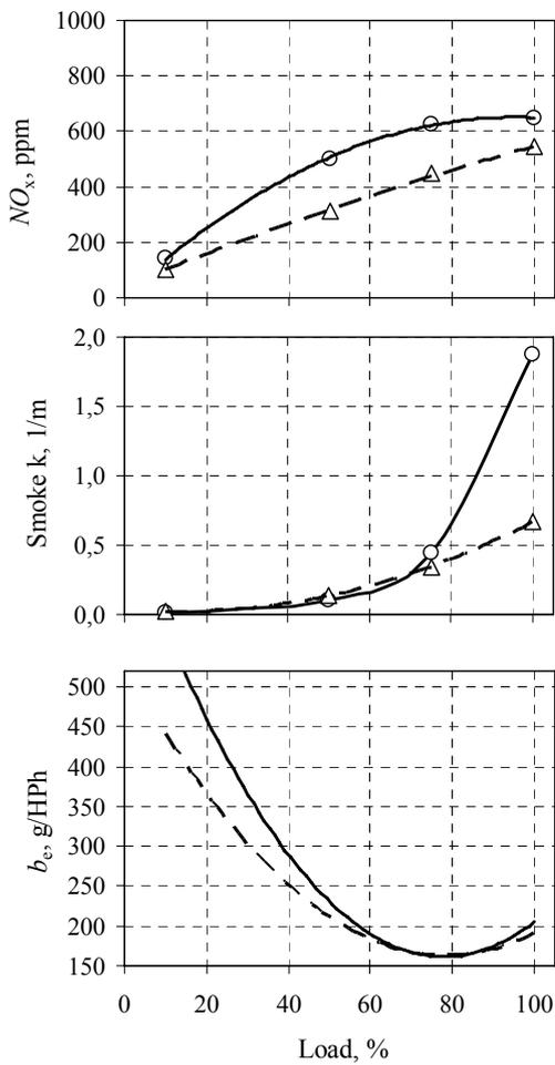
**Figure 6.** Comparison of load characteristics of 4 cylinders naturally aspirated diesel engines with different CCs
