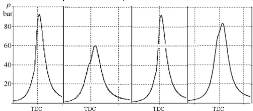
**Figure 4. Theoretical indicator diagrams of different version diesel engines.**
