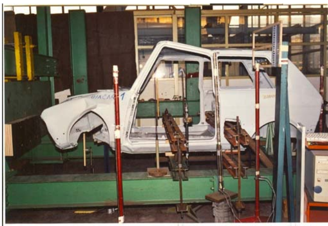
Fig. 11 Car body appearance after quasi-static test
