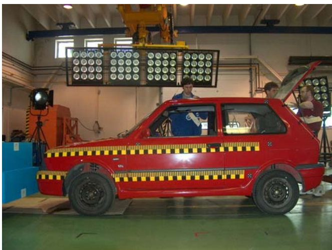
Fig. 12 Impact test conditions according to ECE 94 in longitudinal direction
