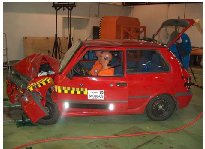
Fig. 14 vehicle appearance after the test according to ECE 94
