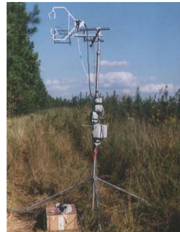
Figure 5. Simple configuration of automated meteorology station
