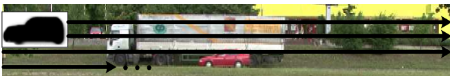
Fig.7 Illustration of the idea of the sliding mask approach – only the values under the black part of the mask are taken into consideration for the specified position of the mask.
