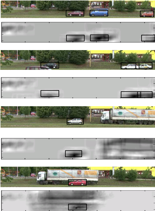
Fig.10 Illustration of the example results of detection based on Euclidean distance in the RGB colour space.
