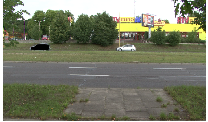
Fig.2 Example frame with the vehicle's model (pattern) marked as the black shape
