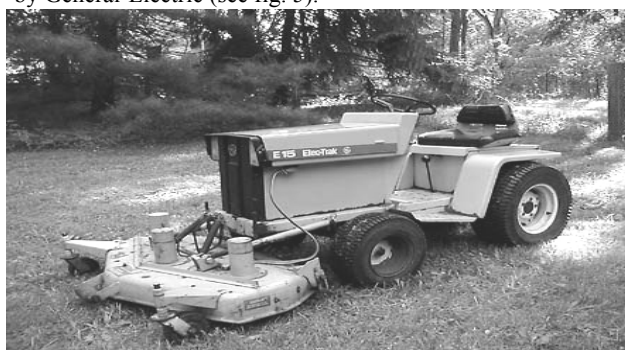
Figure 5. –Electric mini-tractor Elec-Trak
