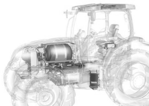
Figure 7. – Prototype tractor with hydrogen fuel cell, NewHolland NH2.
