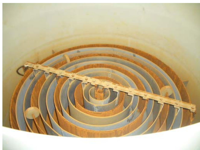
Fig. 1 Arrangement and connection of electrodes in the electrolytic water cleaner (Remark: one of alternatives)
