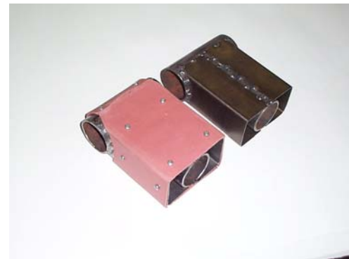
Figure 4. Reinforcement (with and without Betacam mass)
