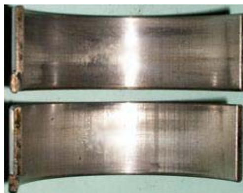
Figure 8. Plain bearing liners of motormixer ABC-7DA bearing roller after 1920-hours operation
