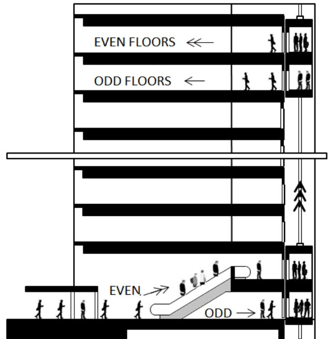
Fig.4 Sectional rendering of double deck elevators
