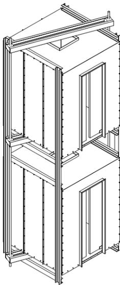
Fig.6 Design of the double-deck elevator car
