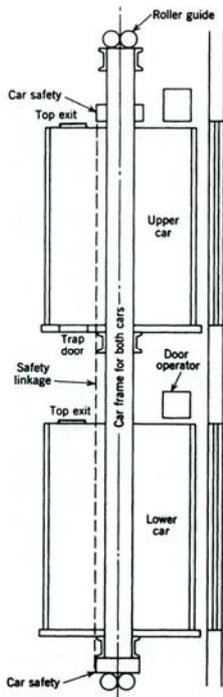
Fig.5 Double-decked elevator car [11]
