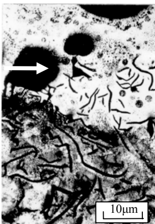
Fig. 7 Gas inclusions and craters due to the graphite evaporating (SCH20, N_s=2.5*10^3 w/cm 2 , \tau=4*10^{-2} s).
