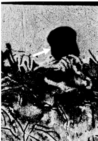
Fig.4 Non-compactness in the bottom of the melted pool due to the partial evaporating of the graphite inclusion. (SCh15, N_s=1.9 \cdot 10^4 \text{ w/cm}^2 , E_v=1.58 \cdot 10^4 \text{ J/cm}^3 ).
